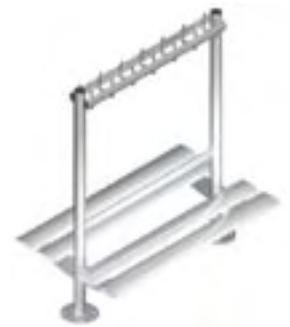
code EL1 double width, island bench with reverse hooks. Free standing units and wall fixed benches require solid floors/walls fixed with Hilti resin type fixings. height 1770 depth 930mm
