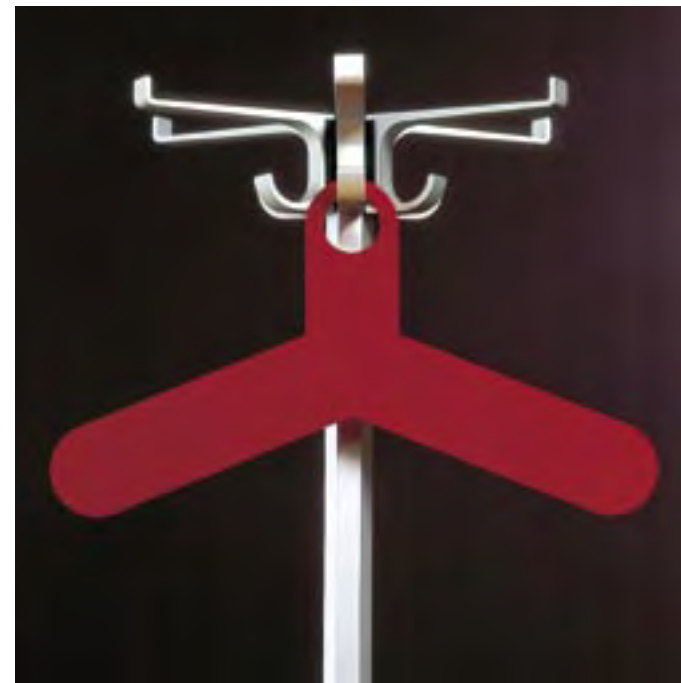
code hat and coat stand VHS The hat and coat stand consists of six aluminium hat and coat hooks fitted to a central aluminium column with an umbrella retaining ring and a drip tray built into the black ABS base cover. The heavy mild steel base ensures excellent stability. The product can be finished powder coated in colour combinations from the full RAL range, or satin anodised.
